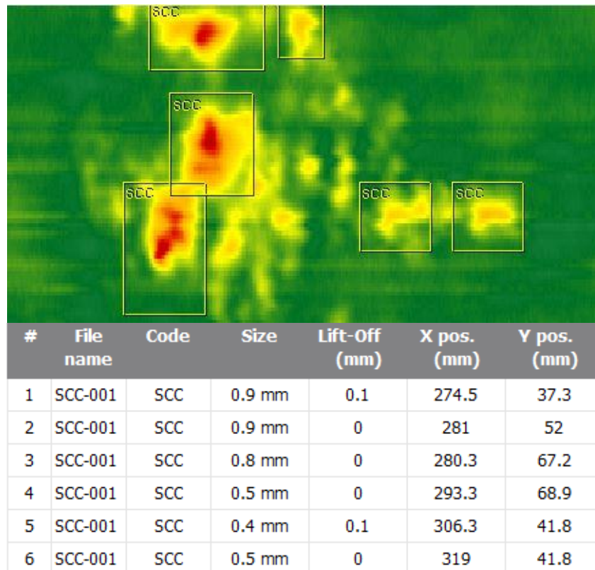
Figure 103. Summary table displayed on the first page of the report, containing information about all the defects that were reported in the current inspection. This is usually followed by individual screenshots and information of all the reported defects.
