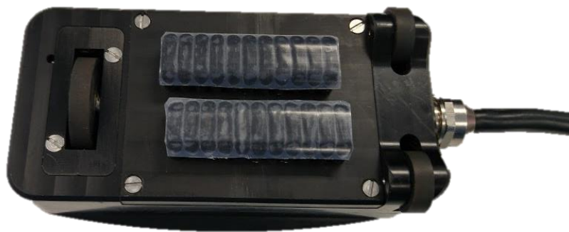
Figure 70. Protective tape applied on probe active area
