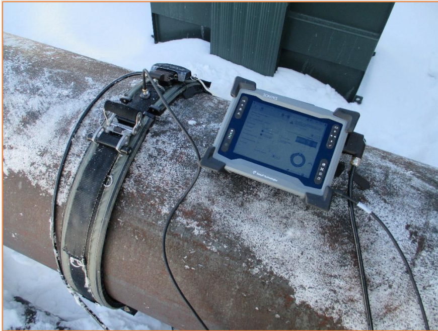
Figure 8: A 36" link-up combination with a Sonyks instrument connected
