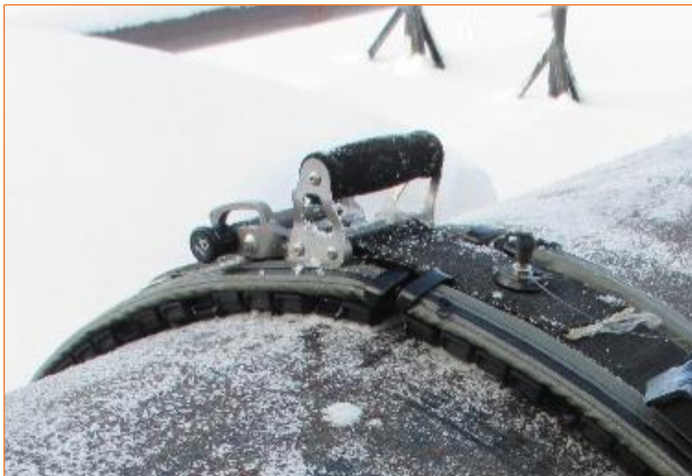
Figure 6: A correctly mounted link-up configuration (note that the webbing is locked via the over-centre clasp and the collar gap has been minimised)
